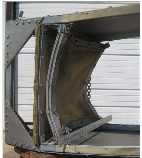
Figure 6. Post-test image of multi-shock shield. Kevlar rear walls are intact (no complete penetration).
