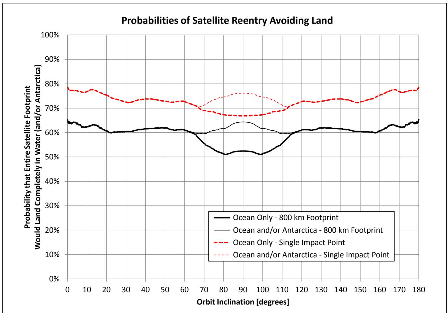
This chart shows the probability that a reentering object will land completely in water as a function of orbit inclination. The black solid curves are computed assuming an 800 km-long reentry footprint. The red dotted curves are for a single object point reentry. In both cases, the effects of the continent of Antarctica are shown by showing the curve if Antarctica were considered “water.”
