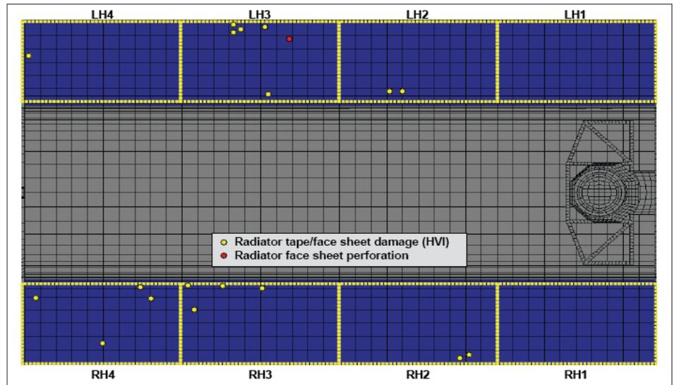
Figure 3. STS-114 payload bay door radiator impact map.
