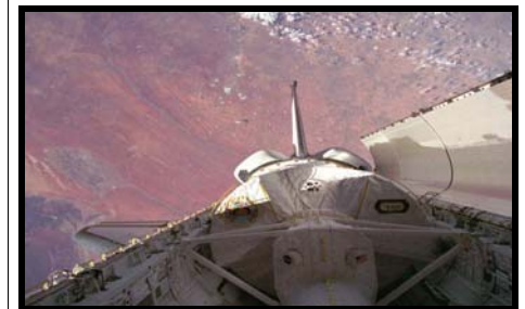
Figure 2. STS-73 mission photograph (with Earth in the background) illustrating the partially open position of the port side cargo bay door. With the door in this position the cargo bay is more protected from hypervelocity impacts.
