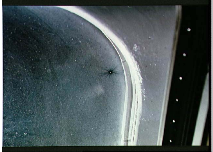
Figure 6. Optical photograph illustrating the hypervelocity impact crater damage site on window #1, taken on orbit.
