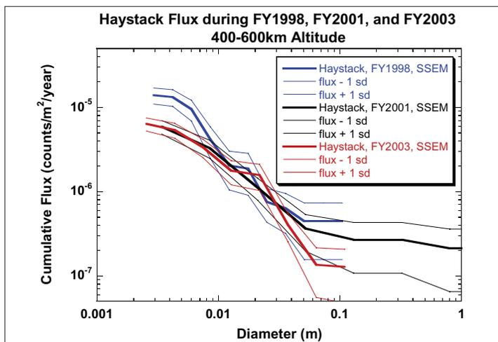
Figure 2. The debris flux versus diameter at 400 km to 600 km for Haystack 75° elevation, east pointing measurements during FY1998, 2001, and 2003.
