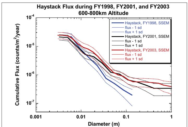
Figure 3. The debris flux versus diameter at 600 km to 800 km for Haystack 75° elevation, east pointing measurements during FY1998, 2001, and 2003.
