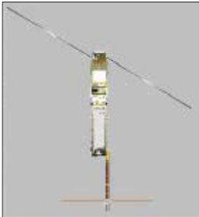
Figure 2. Side view of FORMOSAT III to illustrate the solar panel orientation to the spacecraft body.
