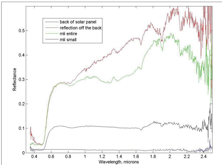
Figure 3. Reflectance spectra of the side of the spacecraft due to terminator lighting. The blue line is the back of the solar panels with direct lighting, the black line is the spectrum of a small piece of MLI, the green line is a larger section of MLI, and the red line is the reflection off the back of the solar panel with side lighting.
