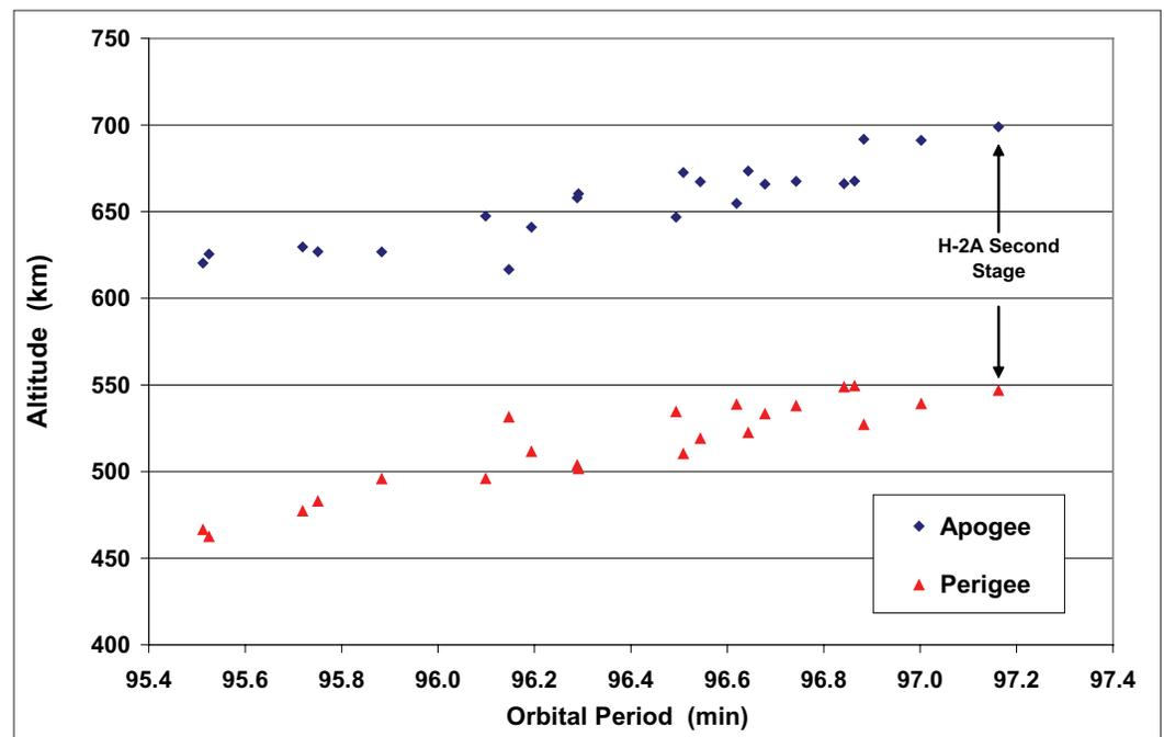
Figure 1. Orbits of the ALOS-1 H-2A second stage and its debris on 9 September 2006.
