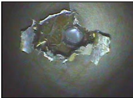
Figure 3. Exit hole in the rear facesheet of the radiator panel.
