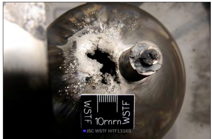
Figure 5. ISS Ni-H 2 cell hypervelocity test damage/perforations (on the left) Test HITF13144, 5.0-mm aluminum spherical projectile at 6.66 km/s and (on the right) HITF13165, 3.8-mm steel spherical projectile at 6.87 km/s.
