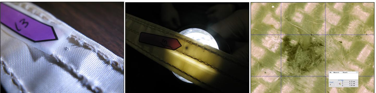
Figure 5. An impact damage (no.13) that was found on one of the hold-down straps. This damage is shown in front-light on left, back-light in middle, and through the microscope on right. The hole diameter in the outer beta-cloth layer was 0.75 mm although the dark zone in the back-lighted photo extended well beyond the hole dimensions.
