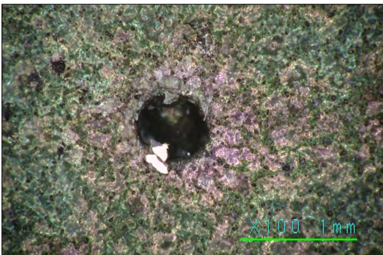
Figure 4. Field imagery of ROI #20, feature size = 0.63 x 0.56 mm, depth = 0.54 mm.
