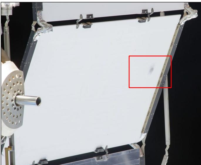
Figure 3. Damage on opposite side of panel.
