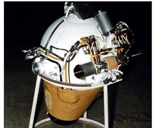
Figure 1. A SOZ unit with its 11D79 engine. Photo credit: RKK Energia/Kosmonavtika.com.
