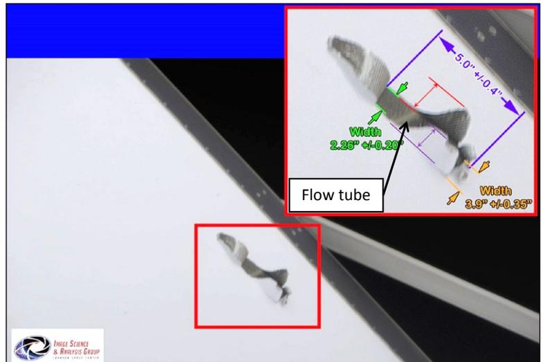
Figure 2. Close-up of exit damage.
