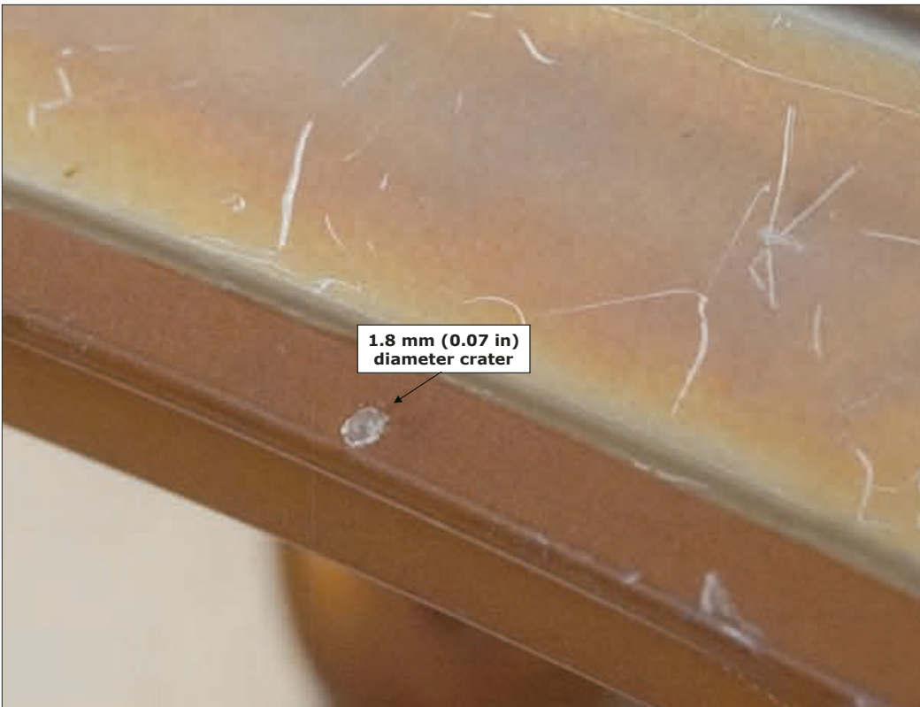
Figure 2. Detail of MMOD impact on airlock hand rail.
