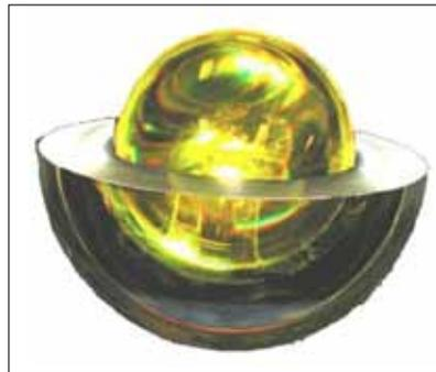
*Cut-away to show the construction of the BLITS satellite.*
