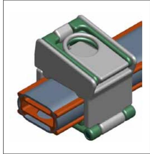
Figure 7. Example of clamp tool to mitigate MMOD damage to handrails.
