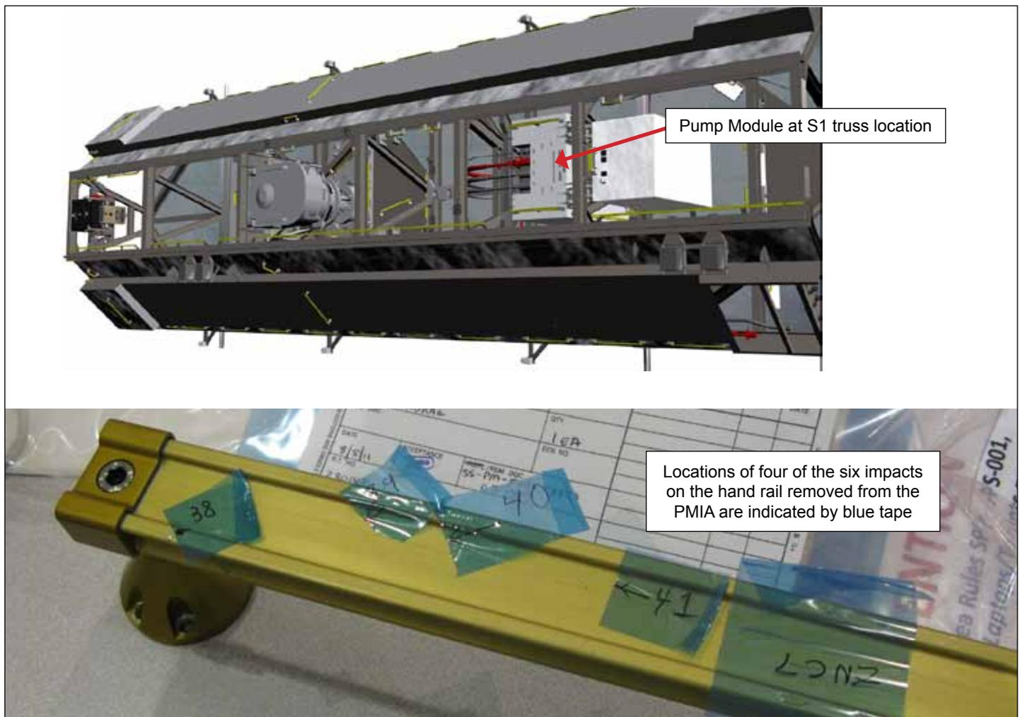
Figure 2a (top). Location of the ISS Pump Module Integrated Assembly (PMIA) on the ISS.
