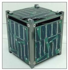
Figure 1. AubieSat 1, a cubesat from Auburn University, which was one of six smallsats launched with the NPP spacecraft.
