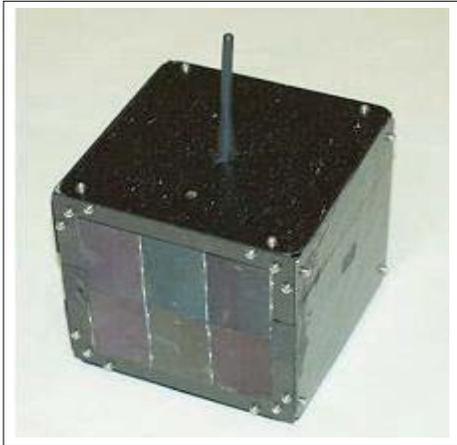
Figure 1. The target microsatellite before the impact experiment.
