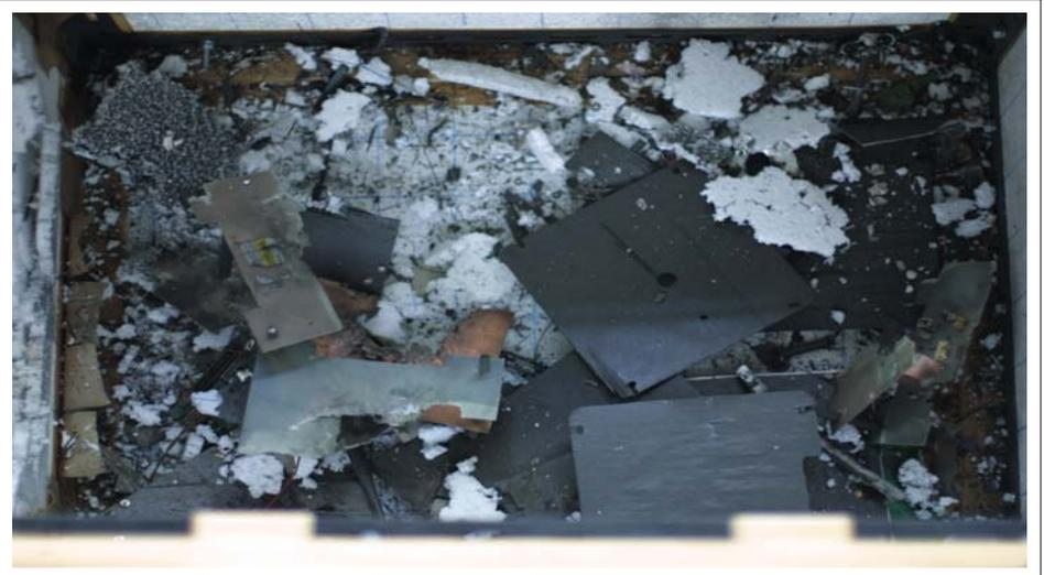
Figure 2. Fragmentation of the micro satellite right after the low-velocity impact. Pieces were mixed with white catch foams from the interior of the test chamber.
