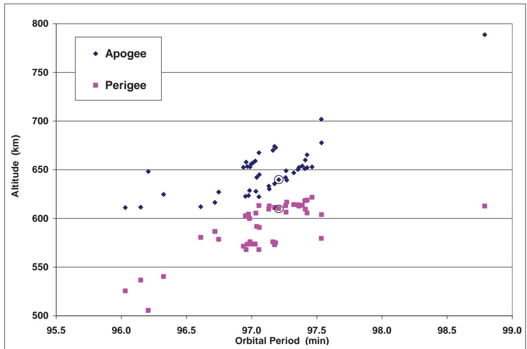
Debris cloud (44 pieces) of the Tsyklon third stage six days after it broke-up on 4 May 2006. The main remnant of the stage is highlighted with circles.
