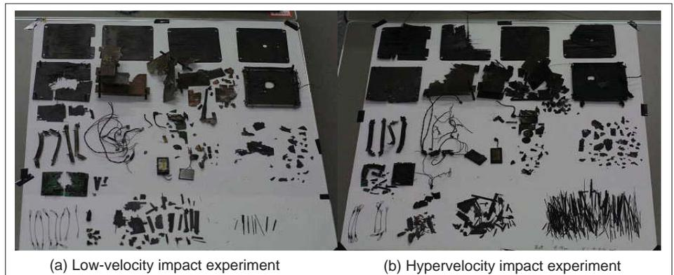
Figure 3. Comparison of fragments from low- and hyper-velocity impact experiments.
