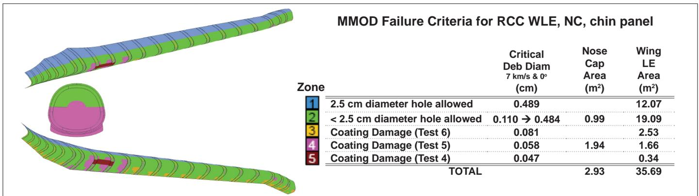
Figure 4. RCC failure criteria and critical particle size.
